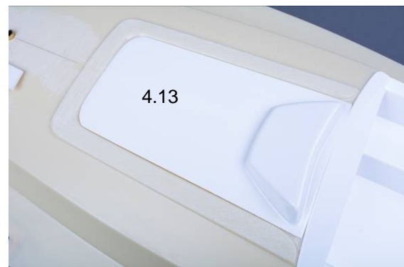
Fig. fitting the sliding hatch
