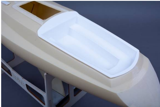
Fig. cockpit fitted in hull
