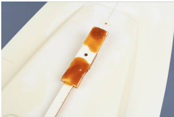
Fig. front reinforcement board with nut M 3 and eyebolt M 3
