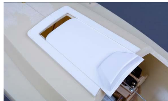
Fig. glued frame, fit sliding hatch
